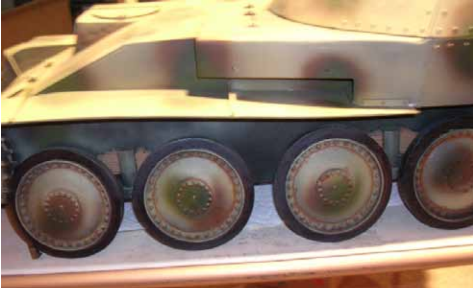
Re-pinned track and repaired wheels, notice the return roller that was added.
